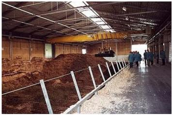
large biological baby food factory. The plant supplies 6.1MW electricity for the grid and the calorific value of the fuel is 9.07 MJ/kg (moisture content 45%).<sup>5</sup>
